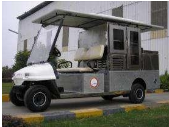
Maini F&B buggies at Bangalore Railway station. With Freezer, Chiller, Warmer, Vending machine & Juicer
